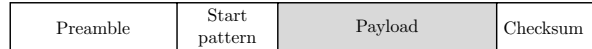
Figure 3: General packet structure of a rolling code. Gray background indicates that the part is either encrypted or authenticated.
